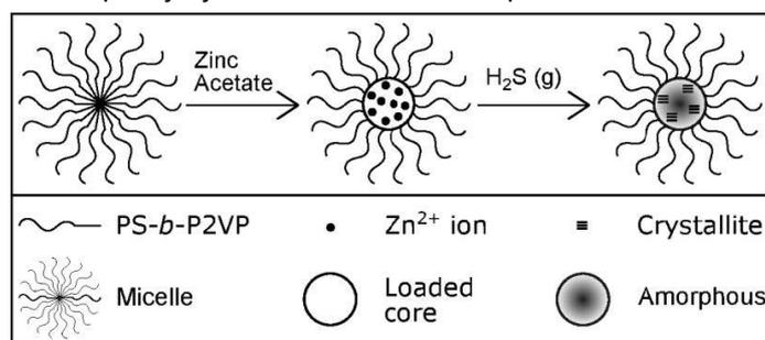
Scheme 1. Schematic showing the mechanism of ZnS nanoparticle synthesis: 1) Zn<sup>2+</sup> ion encapsulation within core of micelles, 2) Treatment with H<sub>2</sub>S generated *in-situ* and 3) Formation of single ZnS nanoparticle with composite sub-structure in core of micelles
